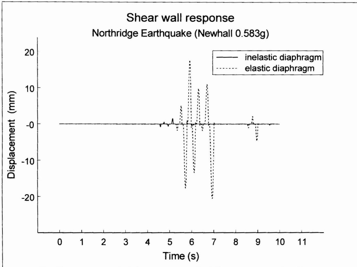
Figure 6: Comparison of end-wall response considering elastic or inelastic wood floor diaphragms
